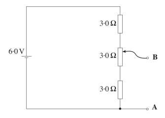
(i) Three  $3.0\Omega$  resistors are connected as shown across a battery of negligible internal resistance. The middle resistor is fitted with a sliding contact as shown in the top diagram. Calculate
